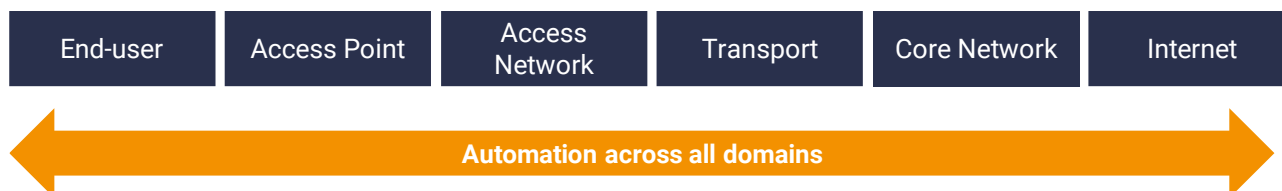
Figure 6: E2E automation can alternatively be defined as automation across different physical infrastructure layers
